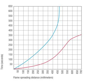
Class 1 Fire reaction chart for coating system RAF-ATB at 520 g/sqm of products.
